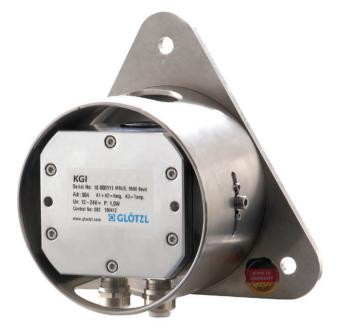
The KGI Tiltmeter is a high-precision instrument for permanent inclination monitoring of structures such as dams, bridges and buildings. Its robust housing makes the KGI ideal for the harsh conditions on construction sites. Even more characteristic and a great advantage is the housing with its cardanic/gimbal bearing system. This design ensures an easy and rapid installation and a precise zero-orientation at the same time.
