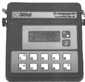
Portable readout unit with simple ring memory for battery operation, type KMG 06-D
